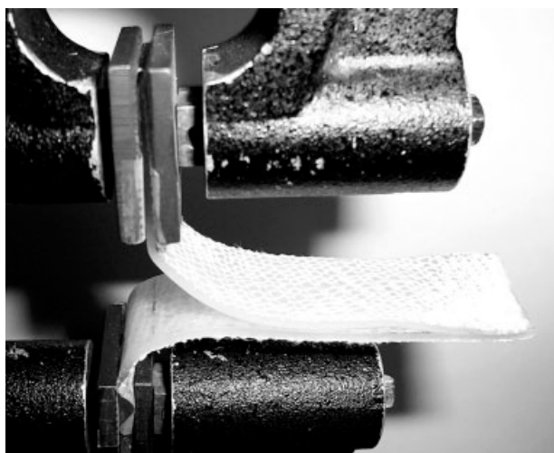
Figure 1 Picture showing a polymer/adhesive/polymer joint in a T-peel test.
